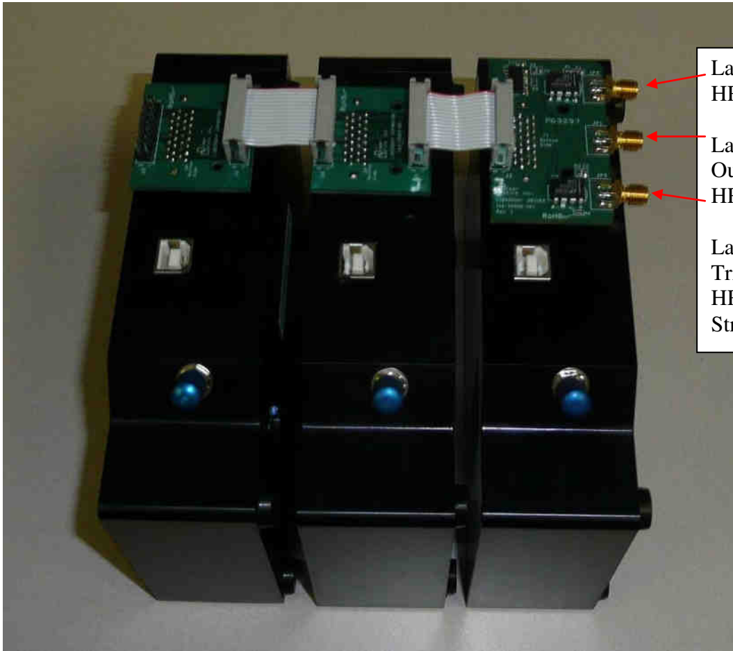
3-channel HR2000+ LIBS setup
